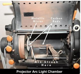
the beginning of the evening, the projectionist had reel #1 loaded on projector #1 and reel #2 on projector #2. An arc was struck on projector #1 and a switch was flipped to start the projector's motor and cause film to advance through the projector. After the film leader passed and the opening frame bearing the studio's trademark (MGM, 20th Centu-Fox, Columbia, reached the projection port, the douser was activated, and the opening frame appeared on the screen.
